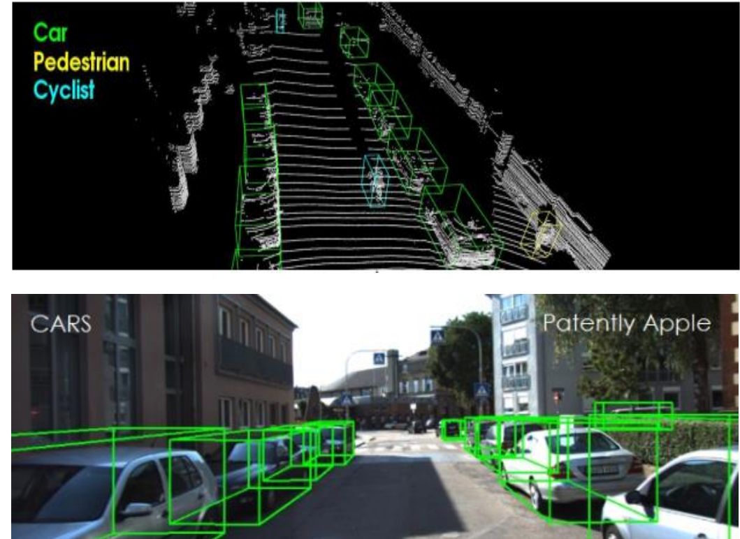
Figure 2. Top: 3D boxes detected in Bird's view image. Bottom: 3D boxes detected in 3D RGB image.
